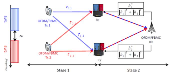
Fig. 8: Cooperative relay for asynchronous multiuser transmission.
