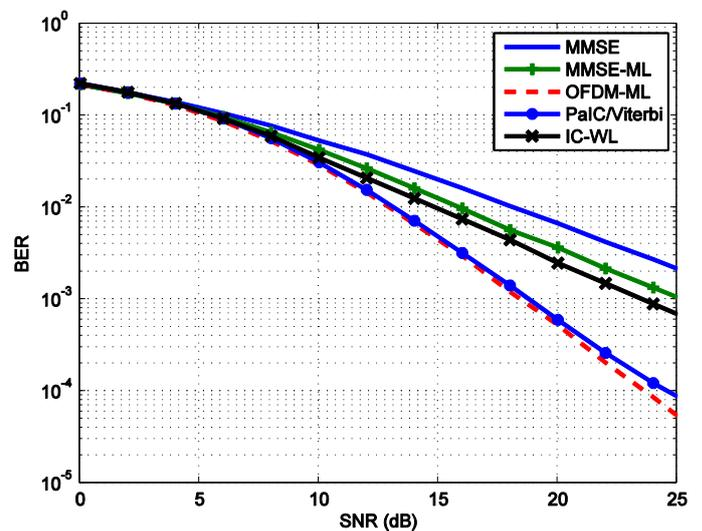
Fig. 1: BER performance comparison of different interference cancellation receivers
