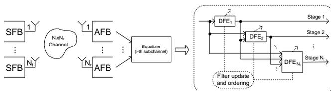
Fig. 2: proposed adaptive equalization of MIMO FBMC systems
