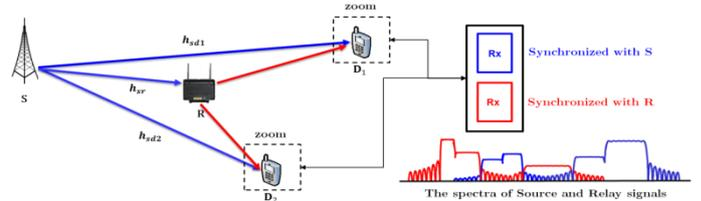
Fig. 7 : structure of the DF-relayed system
