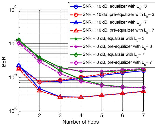
Fig. 5: Comparison of the BER performance in case of SNR = 0 dB and SNR = 10 dB for the FBMC/OQAM based multi-hop relaying network where a multi-tap equalizer or pre-equalizer is employed.
